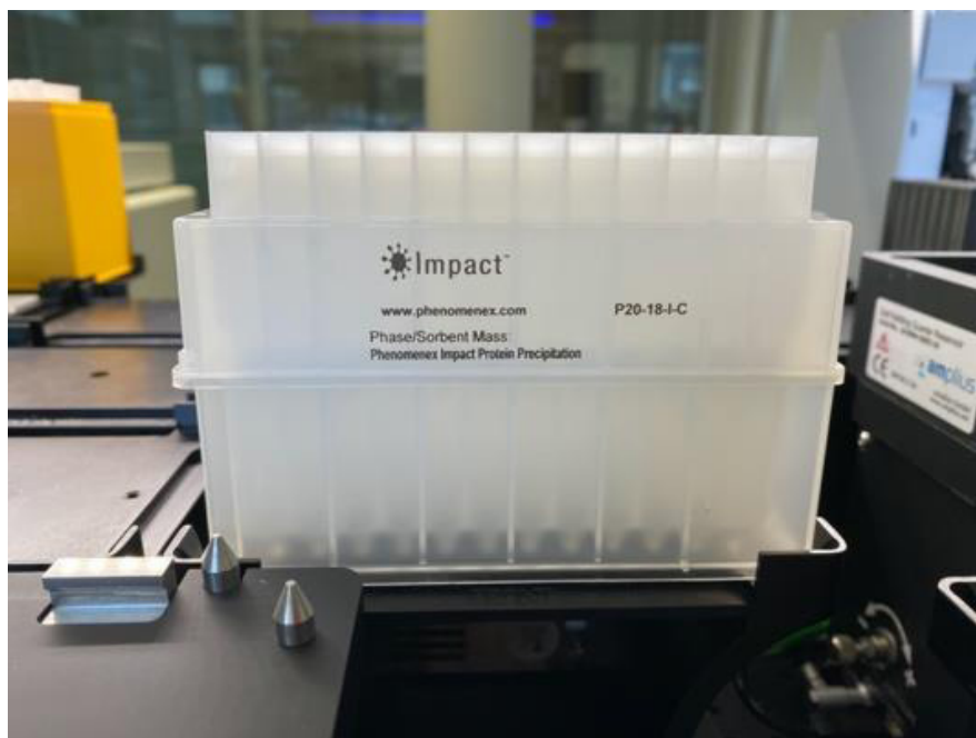
Figure 1. Impact protein precipitation plate (Phenomenex, Torrance, US) with a deep well collecting plate on the Biomek i7 hybrid deck
